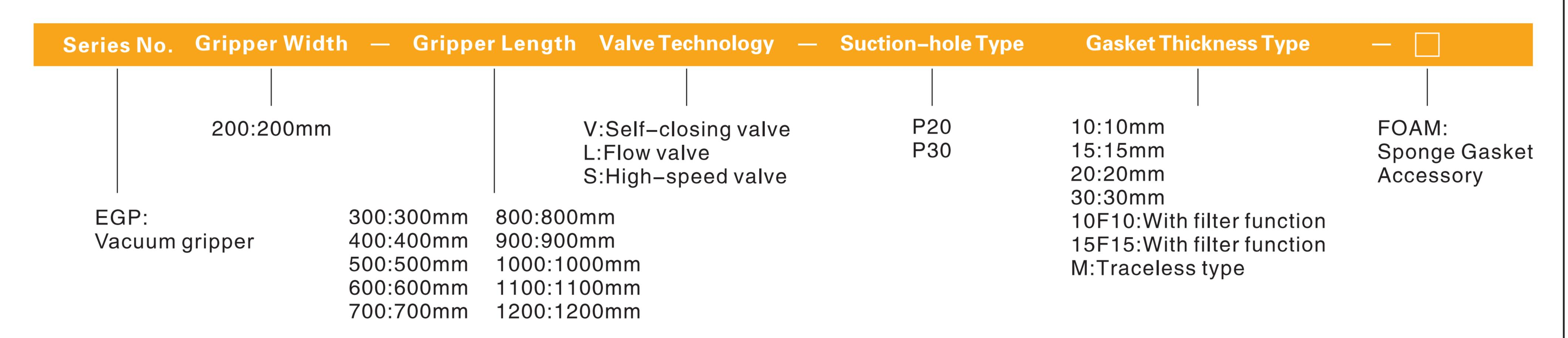
Order Example: EGP series vacuum gripper, gripper width 200mm, gripper length 1000mm, self-closing valve, suctioin-hole type P20, gasket thickness 15mm, sponge gasket accessory. EPR code is: EGP200-1000V-P2015-FOAM
